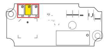
The device is now moved to its limit position wherein the core rod is moved to one of the end positions of the measuring range. In the inner end position (pushed in / fully retracted) the amplifier is adjusted with the sensitivity potentiometer "AM" to the desired lower value, typically 4 mA. Simultaneously the outer end position (pulled out / fully extracted) is adjusted to the upper value, typically 20 mA.
