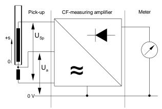
modulated output signal U<sub>a</sub> and converts it to an easy-to-process DC signal (e.g. 0 ... 10 V).
